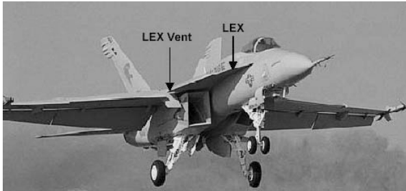
Fig. 1 F/A-18E Super Hornet in approach configuration with the LEX vents open.
